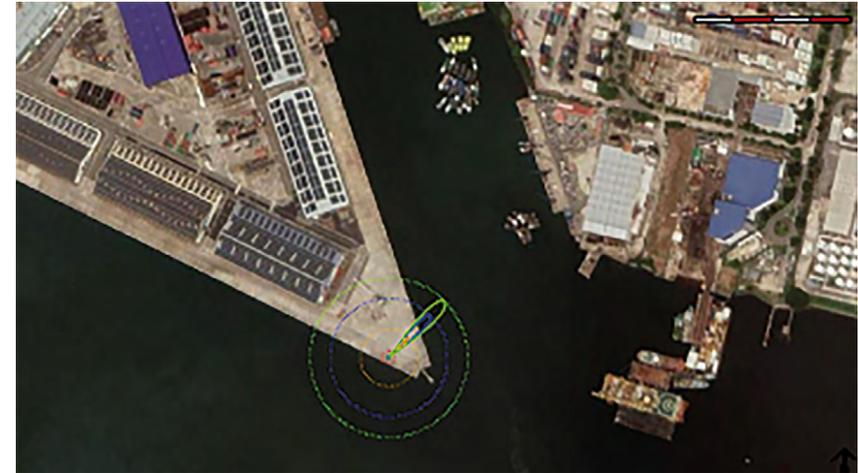
Figure 4.13 Lethality footprints at 0.5 m for truck-to-ship bunkering scenario B
