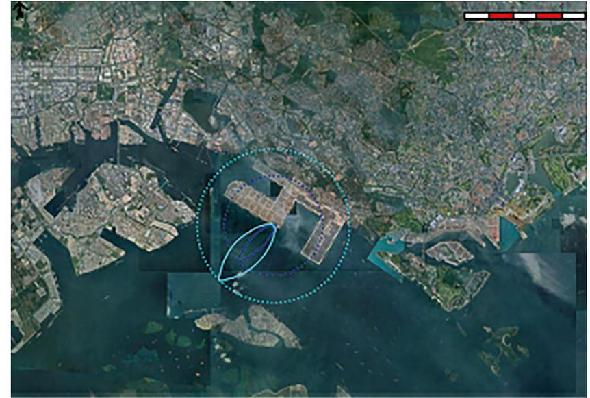
Figure 4.19 Maximum cloud footprints for SIMOPS scenario D (dispersion over the sea)
