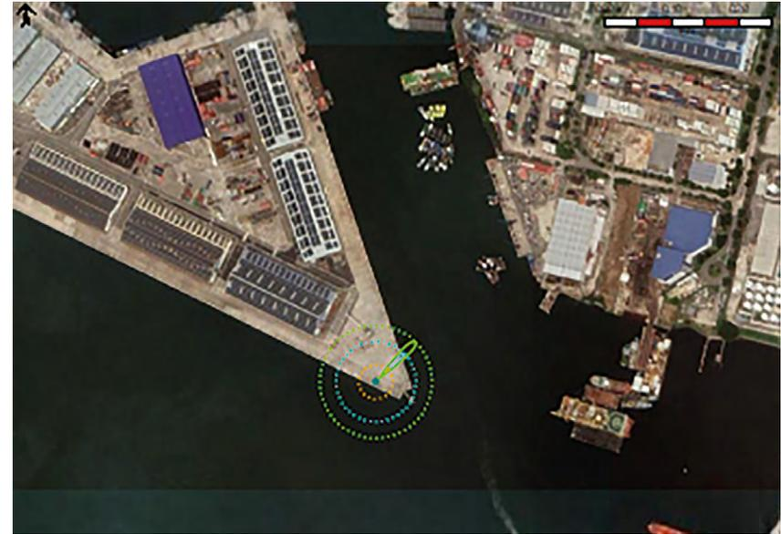
Figure 4.12 Lethality footprints at 1.5 m for truck-to-ship bunkering scenario B
