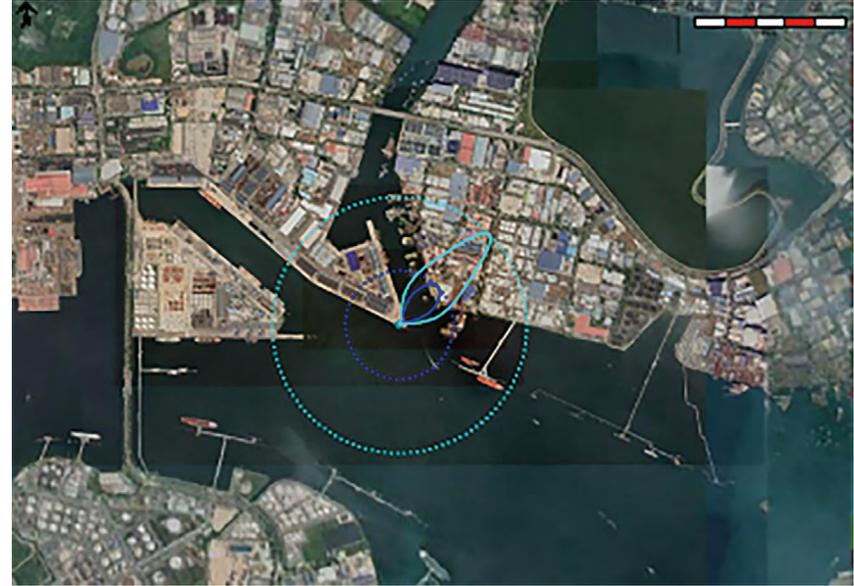
Figure 4.11 Maximum cloud footprints for truck-to-ship bunkering scenario B
