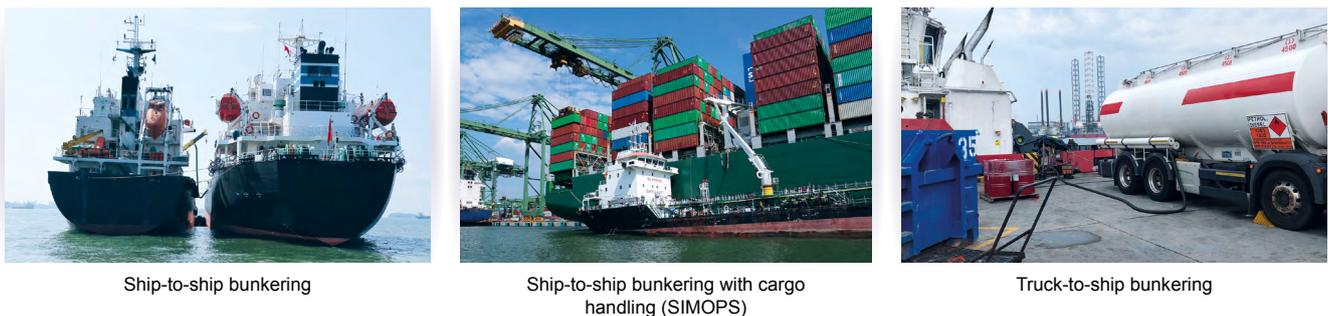
Figure 3.1 Different bunkering modes for conventional marine fuel carried out in Singapore
