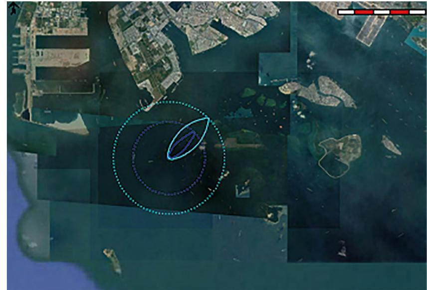
Figure 4.15 Maximum cloud footprints for ship-to-ship bunkering scenario C
